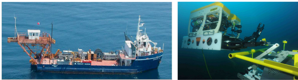
Figure 11. Photograph of the Castor boat, used for the KM3NeT/ORCA string deployment (left). Photograph of the Comex Apache ROV used for the KM3NeT/ORCA string connection (right).
